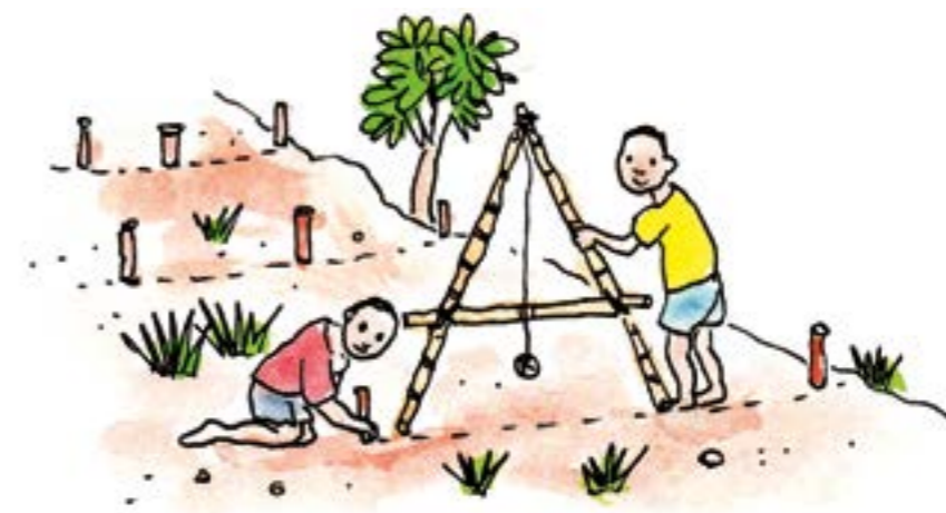
Using an A-frame to measure contours
