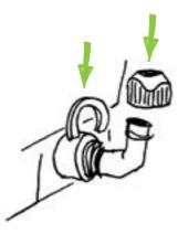
Slide circlip down groove at end of thread to 4 stop outlet from sliding back into the tub.
