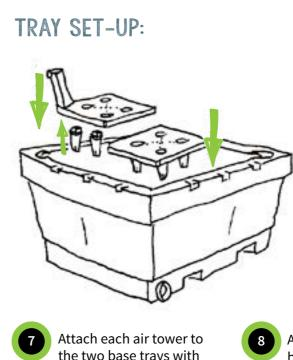
Place tubs close together with outlet 10 stubs facing each other. (Level setter must remain on end tub.)
