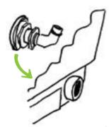
Insert level setter, outlet and seal from the inside of the tub until the thread is fully visible. Straight edges must align.
